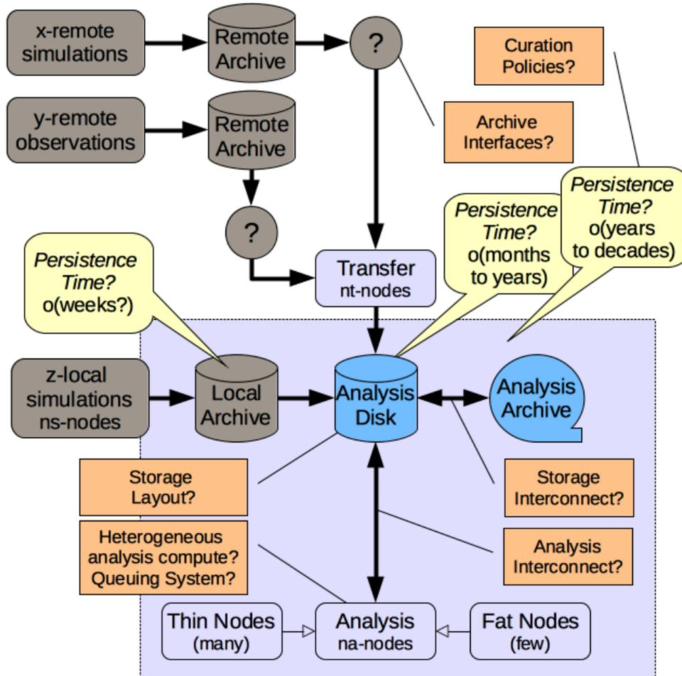
Multiple remote data sources: can't bring the compute to all data, SO: bring all data to one place, and bring the compute to that! (Avoid  $n \times n$  data transfer!)
