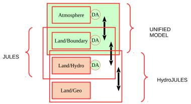
Note expectation that "coupling" may extend through domain of multiple models and doesn't necessarily simply involve exchanging fields.
